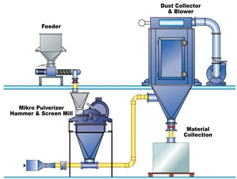
For continuous operation of the Mikro Pulverizer® Hammer & Screen Mill, material can be air conveyed away from the mill and collected in a downstream product collector. The valve you see located in the ductwork at the inlet of the conveying duct under the mill is used to regulate the amount of air pulled through the mill during operation.
