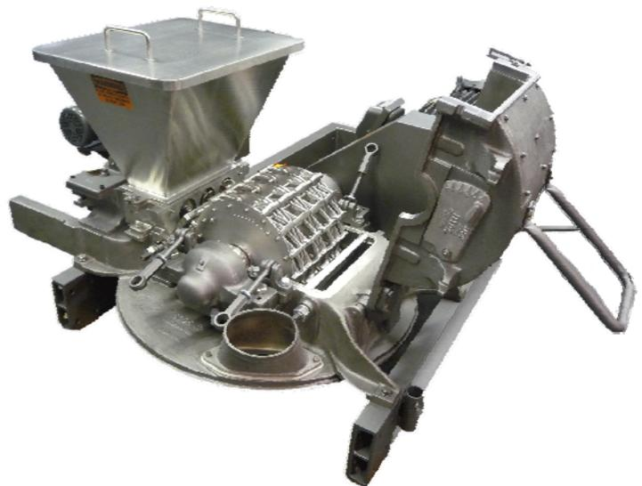
material the mill can process, so heat generation will occur during the milling process and must be considered when designing a system around this type of mill. Air can also be conditioned to provide the appropriate operating temperature for the material being processed.
